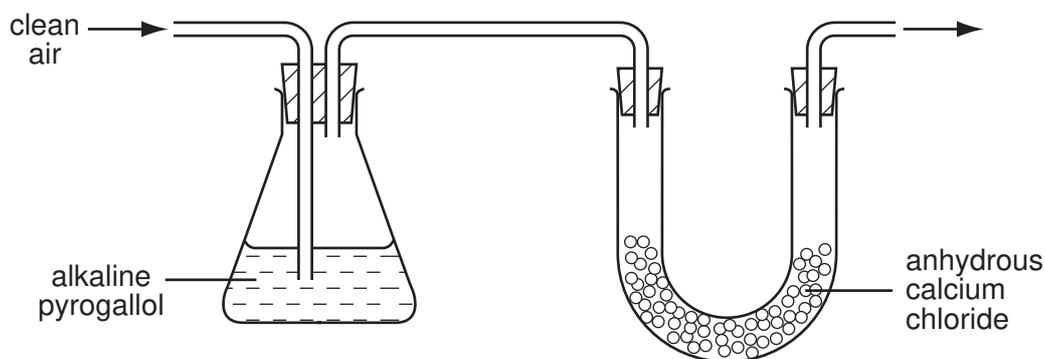
Which gases are present in the air leaving the apparatus?
